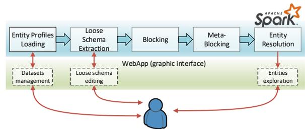
Fig. 3: *Blast* logical architecture.
